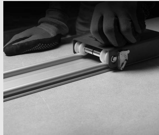
CUTTING DETAIL WITH GUIDE ON SLAB
